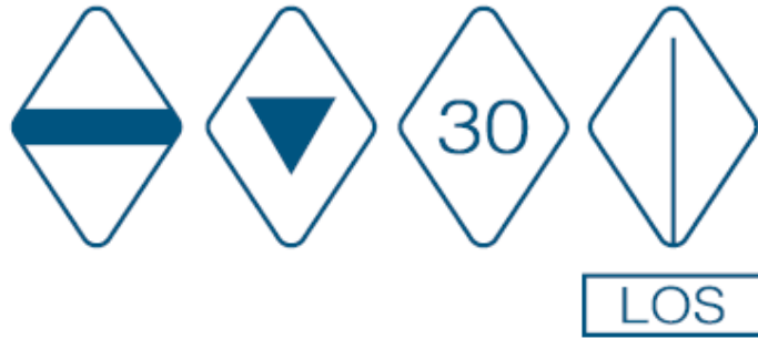
Figure 8: To indicate to tram traffic the requirement to stop, and not to proceed until it is safe to do so
