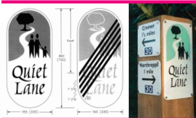
Norfolk Quiet Lane sign, used in conjunction with non-motorised user signs showing distance to next village and cycle route number (see right)
