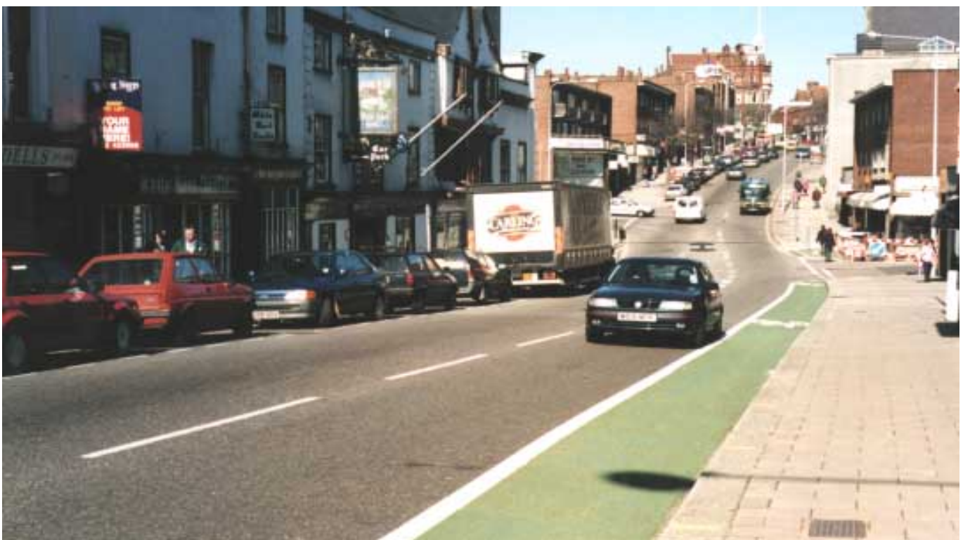
Plate 8 Coloured Surfacing used to Supplement Road Markings for a Cycle Lane
