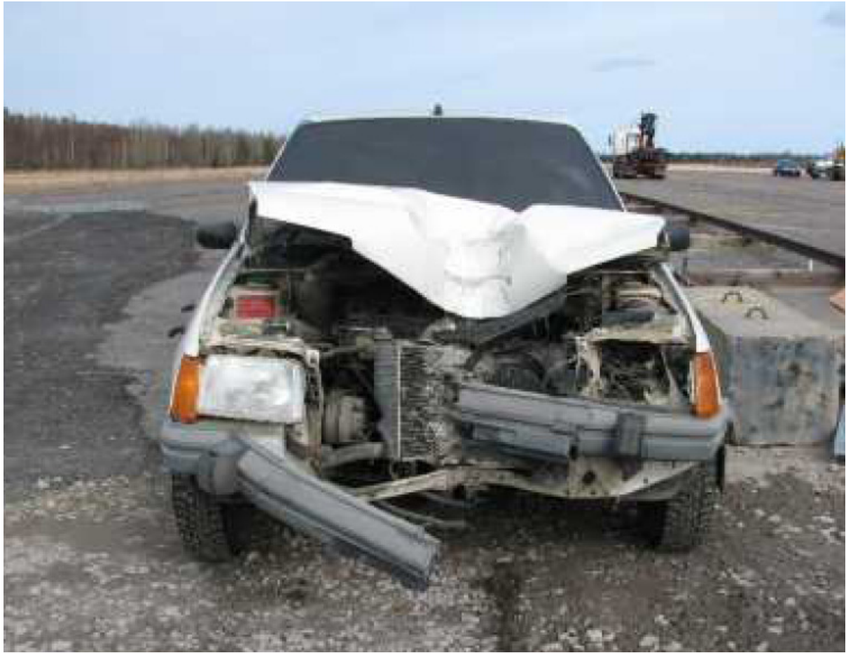
VEHICLE AFTER CRASH TEST(No windscreen or roof damage)
